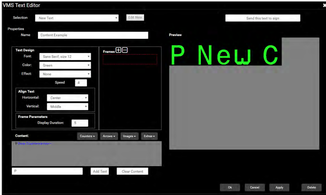
Figure 104: Example of mixed text and content options to display an informative message
